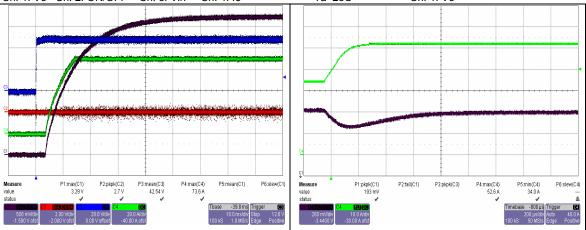
Start-up from Input Voltage Application at Full Load. Ch. 1: Vo Ch. 2: ON/OFF Ch. 3: Vin Ch. 4: Io
